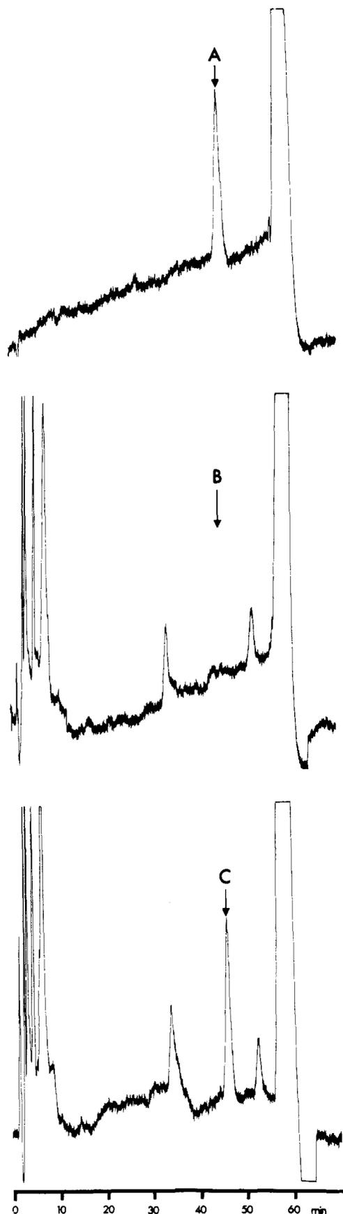
Figure 3. Chromatograms of standard oxime and leaf extracts: (A) standard 1 ppm of oxime; (B) untreated leaf extract after cleanup; (C) combination of (A) plus (B) (1 ppm of oxime prepared in untreated leaf extract after cleanup).
