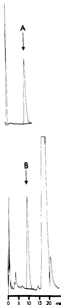
**Figure 2.** Chromatograms of standard oxamyl and seed extract: (A) standard 10 ppm of oxamyl; (B) treated seed extract without cleanup.
