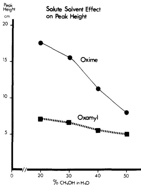
**Figure 1.** Influence of compositions of the mobile phase (volume/volume percent of methanol in the methanol and water system) on peak heights of oxamyl and oxime (Brownlee C-18 column; oxamyl and oxime were both at 4 ppm).
